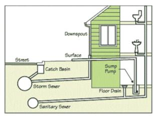
IF your sump pump is pumping directly into a drain in your house it is going into the Sanitary Sewer System...
